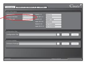
If the Firmware Revision is H, or later, then it is safe to update the Oasis firmware using the OCC App. The Oasis Firmware Update is always delivered in a zipped folder containing the current firmware for all of the Oasis cards and boards. The Firmware Update can be downloaded from any Harris BCD support site. Once downloaded, click the search button \_\_\_\_\_ to open the download
